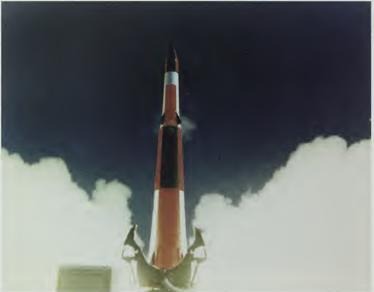
Fig. 5-14. Unlike other theater missile defense systems, the Arrow, which travels at Mach 9, employs a warhead to intercept its targets.
